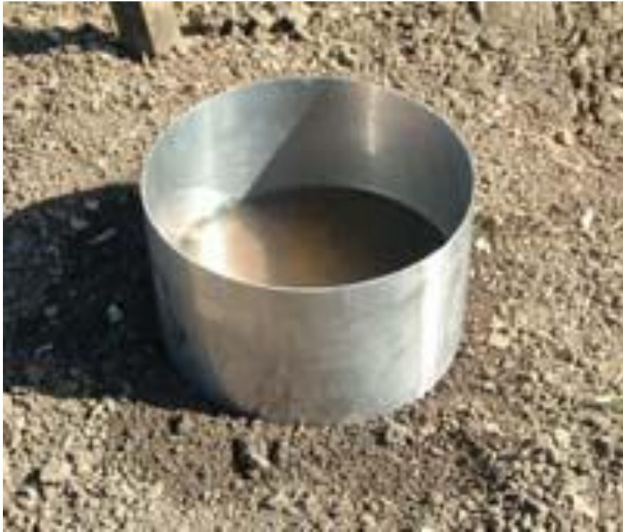
Figure VII.1. Photo of Single Ring Infiltrrometer
