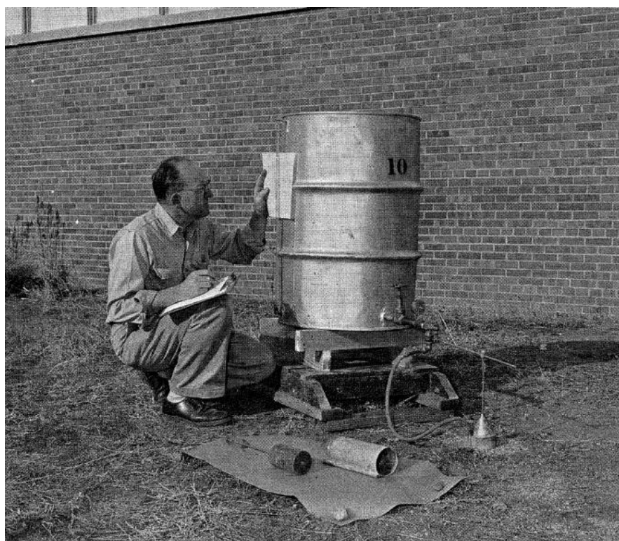
Figure VII.13. Typical Well Permeameter Test Installation
